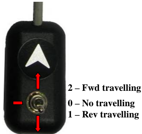
Fig. 9.4 – Movement control device – positions explained.
