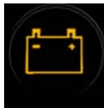
Fig. 3.11 – Power reserve or BMS fault code indicator light.
