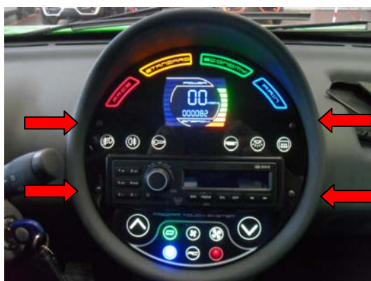
Fig. 10.4 – Touch panel removing.
