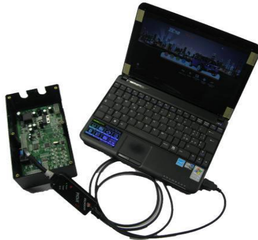
Fig. 6.3 – PICkit 2 programmer plugged in the service PC and in the peripheral device to program (in this photo, the BMS electronic control unit).
