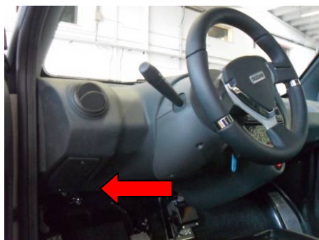
Fig. 10.1 – Main fuses box
