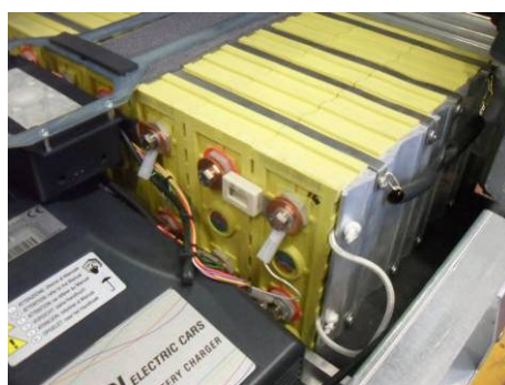
Fig. 10.7 – Battery power line protection
