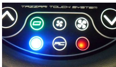
Fig. 4.6 – Tazzari Touch System, Electric heating
