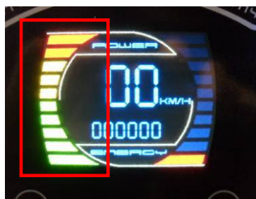
Fig. 4.4 – Tazzari Touch System, Econometer (Power)
