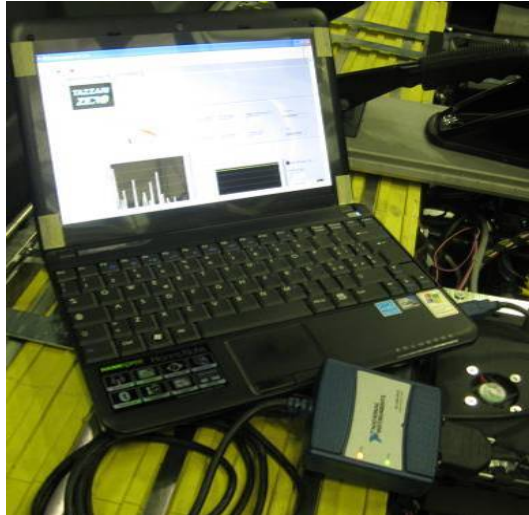
Fig. 5.1 – Service PC connected to CAN to USB Adapter.
