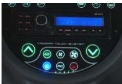
Fig. 4.5 – Tazzari Touch System, Forward/reverse travelling selector
