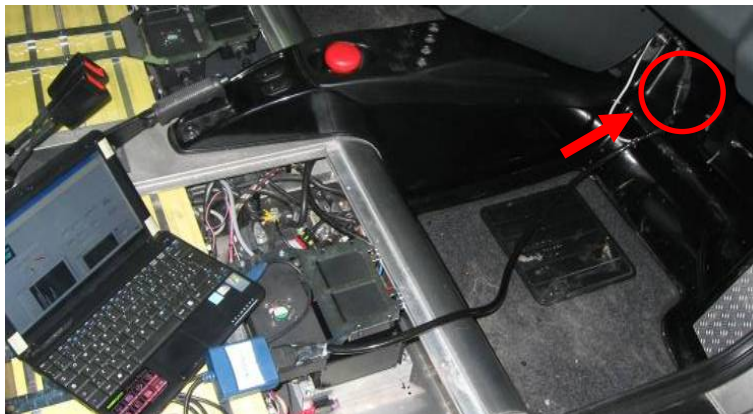
Fig. 5.2 – Service PC connected to the CAN to USB Adapter and to the BMS test socket
