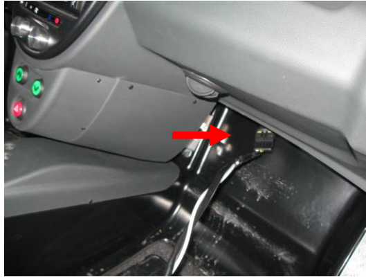
Fig. 4.2 – BMS Console connection to Zero.
