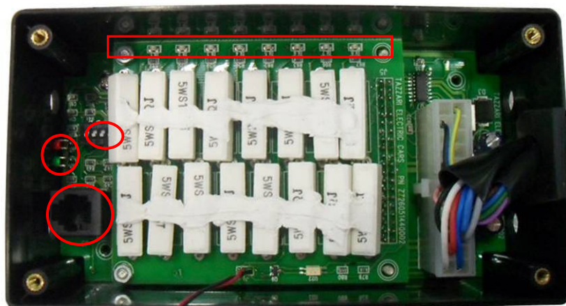
Fig. 3.7 –BMS Modul7Equalizere (with the two LEDS and programming connector circled).
