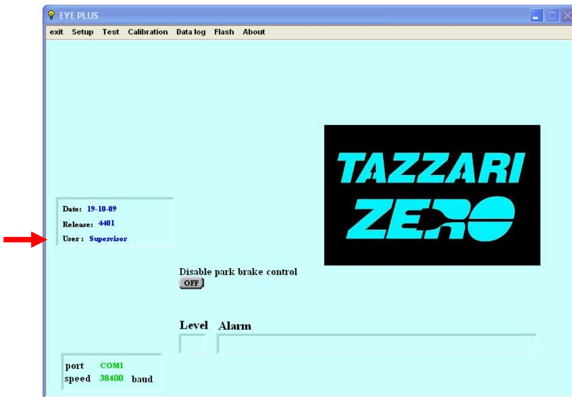
Fig. 3.10 – EyePlus screen – connection to Supervisor mode established -.
